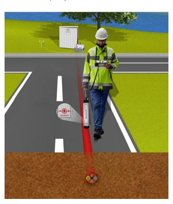
This means that the highly precise receiver is still able to deliver clear results in areas with lines that are routed closely together.
