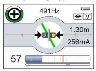
Along with the tracking signal, the new measurement screen provides a clear overview of all relevant information that can be useful in locating the cable or probe.
