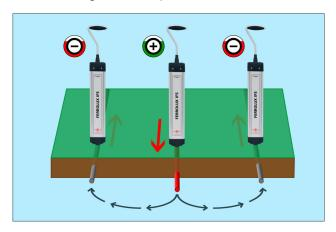
If there are several lines (cables, pipes) located next to each other, it is often difficult to determine which the correct one is. Sometimes the signal from the generator can flow through both lines, but the signal in the lines may be flowing in different directions. With the SignalSelect function, the generator applies a signal that contains directional information. When the device is positioned over the correct cable, a "+" symbol is displayed to facilitate precise identification.
